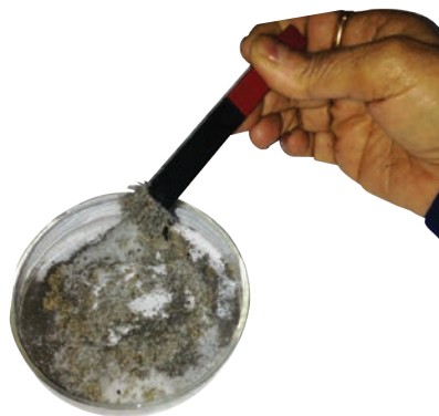
Figure 9.2 Iron filings get attracted towards magnet
