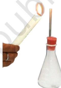
Figure 19.2 Testing hydrogen gas by burning
