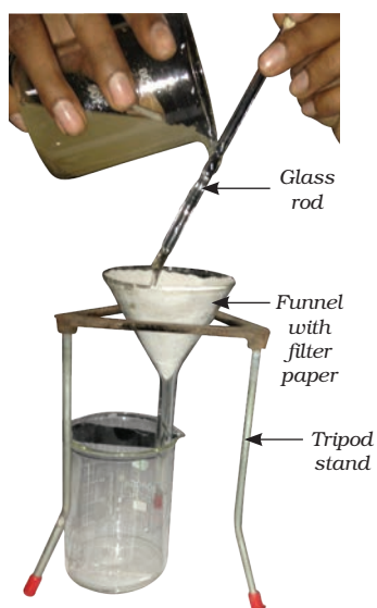
Figure 9.3 Filtration using a filter paper
