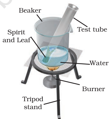
Figure 4.1 Set-up for extraction of chlorophyll
