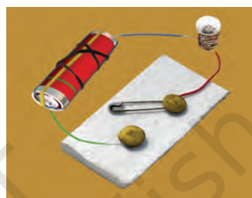
Fig 12.9 An electric circuit with a switch
