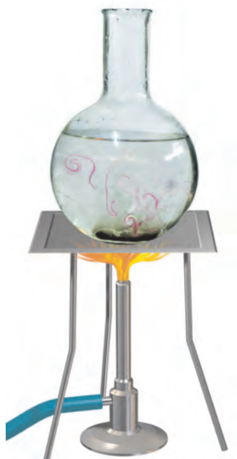
Fig. 4.9 Convection of heat in water
